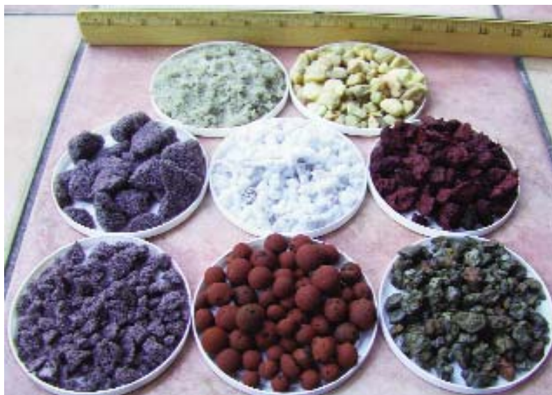
Some examples of media used in semi-hydroponics. Front row, (all left to right): medium grade Growstone, Hydroton, lightweight expanded shale aggregate (LESA). Middle row: coarse Growstone, sponge rock, red lava pebbles. Back row: coarse sand, pea gravel.
