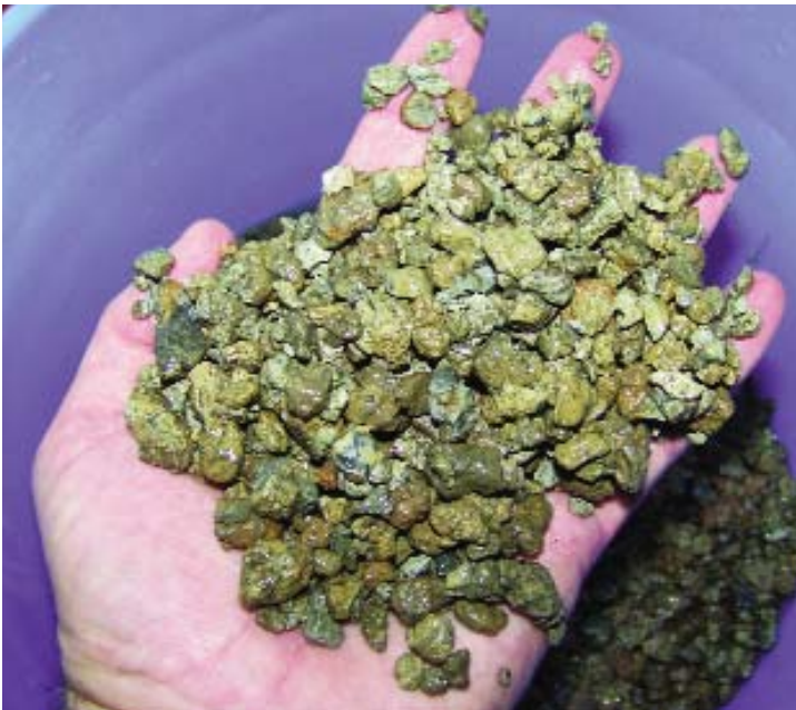
Lightweight expanded shale aggregate, LESA, can have an attractive mix of colors.
