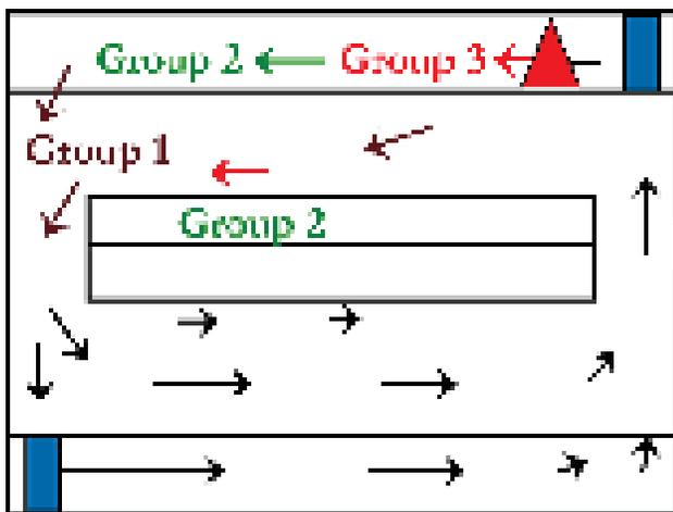
Figure 1. A circular air flow pattern is produced by two large box fans on opposite ends and side of the greenhouse. The hanging partition in the center of the greenhouse for mounted plants also separates the air columns. When the heater is on (red triangle) air moves from the front of the greenhouse toward the back and becomes progressively cooler. Based on the size and make up of our collection there is no need to evenly heat the entire greenhouse.
